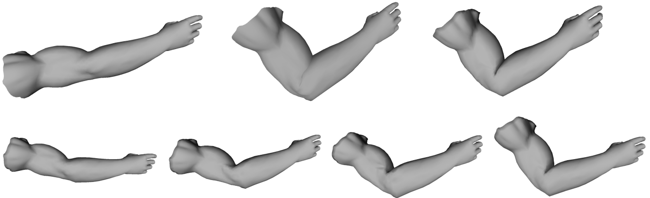
Fig. 3. Using edge-length interpolation to combine skeletal motion and blend shapes for animation. The original arm mesh (upper left) is bent using linear blend skinning, producing a self-intersection (upper middle). The bent arm pose is then cleaned up interactively to remove the self-intersection (upper right). Four intermediate steps of edge-length interpolation between the original straight arm and the cleaned-up bent arm interpolate both the skeleton-derived motion and the edits.
